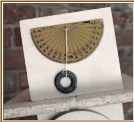
Figure 8. A Home-Made Device for Setting Fretsaw Table Angles
