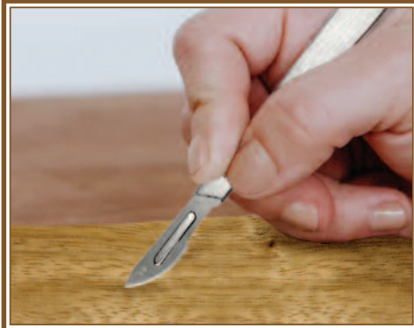
Cutting using the Window method
