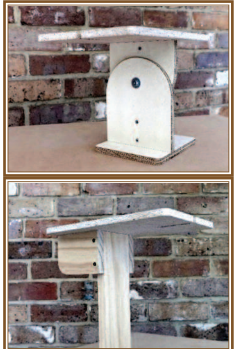
Figure 7. Homemade Fretsaw Tables: Tabletop Version and Vice-Held Version
